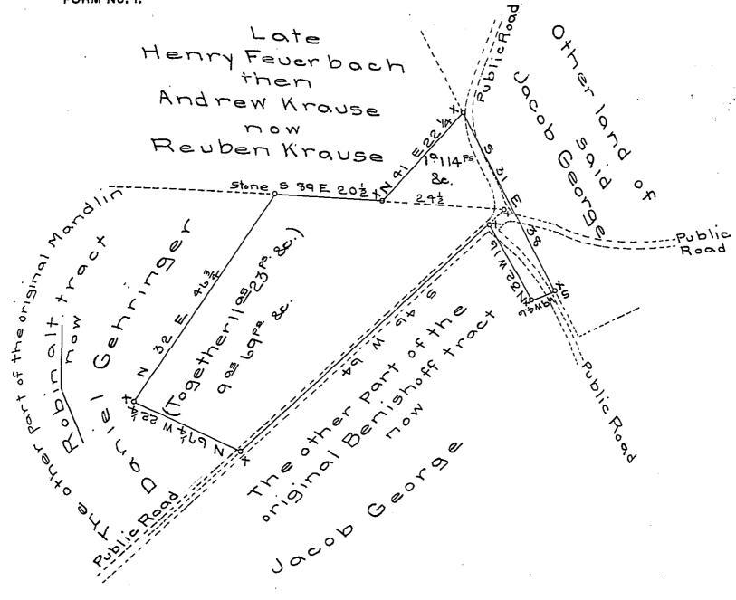
Draft of a tract of land situate in Lowhill town-ship. Le high County containing 112 23 ps and allow-ance of six per cent for roads & Returned for Jacob George this 25" day of Nov. A.D. 1874 the 1914 ps thereof being part of 63 as 142 ps & originally surveyed to Valentine Benishoff by warrant dated April 22 d 1752 and the 9 as 69 ps being part 94 as 148 ps & warrant dated April 11th granted to Mandlin Robenalt
